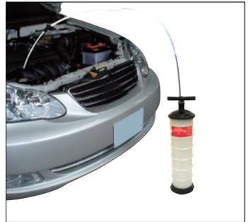
4. After all the oil has been extracted, press the "Release Valve" for at least 5 seconds to release any vacuum formed in the inner pump tube. Remove the extracting tube from the dipstick tube (refit the oil dipstick). Remove the main suction tube from the unit. Slowly pour the used oil into a suitable container and dispose appropriately.
